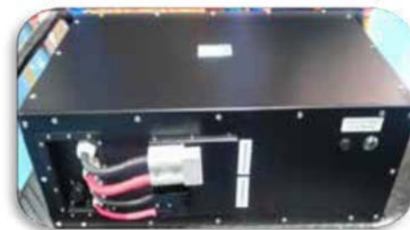
Golf Cart Battery Pack
